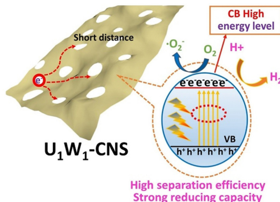
Fig. 10 Schematic illustration of porous GCN. Reprinted with permission from ref. 74 Copyright 2021, Elsevier.
