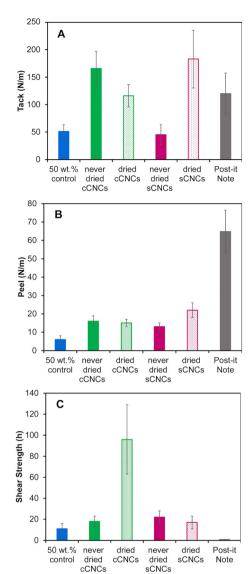
Fig. 4 (A) Tack (B) peel strength and (C) shear strength measurements of latex films with 1 wt% incorporated CNCs having different surface chemistry (carboxylated vs. sulfated) and storage methods (never-dried vs. dried). Error bars represent the standard deviation of  $n \ge 3$  repeats.
