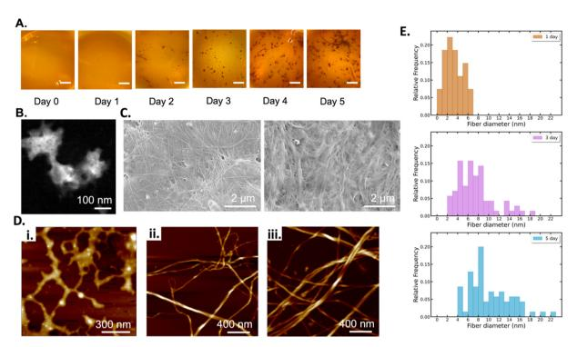
Fig. 2 BC growth at timepoints: 1d, 3d, and 5d: (A) Photographs of the culturing flasks at 24 h timepoints until 5-day (all scale bars are 5 mm). (B) STEM image of BC 1d, (C) SEM images of BC 3d and 5d, (D) AFM images of BC (i) 1d, (ii) 3d and (iii) 5d, and (E) histogram of the fibril diameter distribution for 1d. 3d, and 5d measured in the AFM data.
