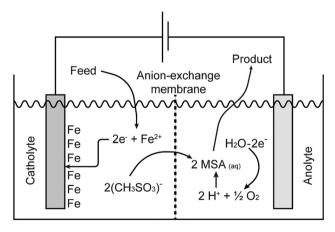
Fig. 17 Divided electrochemical cell for recovery of MSA from a Fe  $(CH_3SO_3)_2$  solution. The cell is divided by an anion-exchange membrane that allows transfer of the MSA anion from the cathode to the anode compartment, where is combines with the protons formed by oxidation of water. Redrawn from ref. 5 with permission from the Royal Society of Chemistry, copyright 1999.
