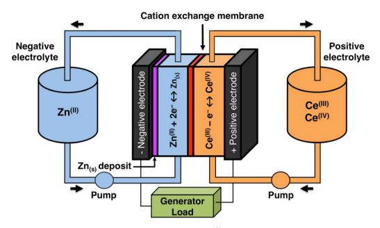
Fig. 16 Diagram of a divided zinc-cerium redox flow battery. Source: wikipedia. 168
