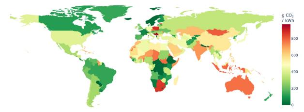
Fig. 2 Average CO<sub>2</sub> emission per produced kW h of electricity based on the international electricity factors of 2023. 121 The energy source of a data center is a crucial factor in determining the environmental burden of computing.
