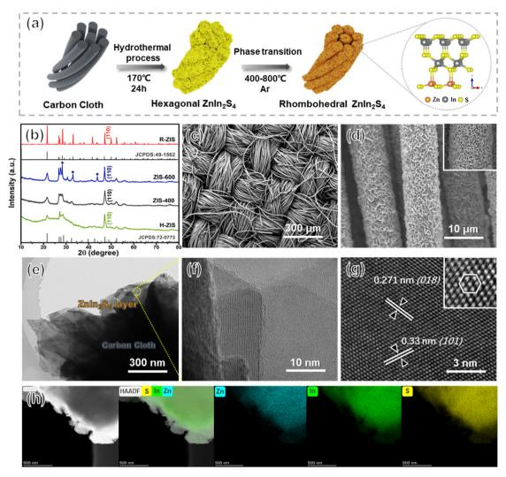
Fig. 2 (a) Preparation of the ZnIn<sub>2</sub>S<sub>4</sub> electrodes through hydrothermal and annealing treatment processes. (b) XRD patterns of the as-prepared H-ZIS, ZIS-400, ZIS-600, and R-ZIS samples and their reference cards. (c and d) FESEM images of the R-ZIS electrode. (e and f) TEM images, (g) HRTEM image, and (h) EDS mappings of the R-ZIS electrode.
