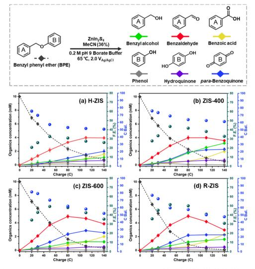
Fig. 4 Kinetic profiles of product distribution during electrolysis on different electrodes: (a) H-ZIS, (b) ZIS-400, (c) ZIS-600, and (d) R-ZIS.
