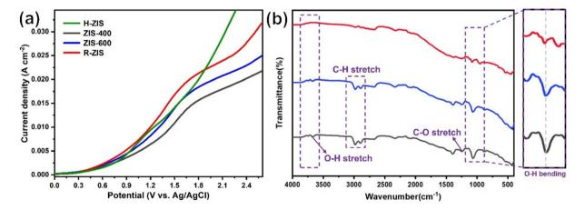
Fig. 5 (a) Linear sweep voltammetry (LSV) curves of BPE on different ZIS electrodes at a scan rate of 50 mV s<sup>-1</sup> in standard reaction conditions. (b) ATR-FTIR spectra of post-reaction tainted carbon cloths after adsorption and oxidation–catalysis reaction of phenol in the R-ZIS electrode. (Red) pristine R-ZIS electrode. (Blue) Adsorption of phenol in open-circuit conditions for 8 h on R-ZIS. (Black) Electrolysis of phenol for 8 h on R-ZIS.
