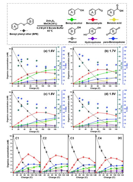
Fig. 6 Electrolysis of BPE using the R-ZIS electrode in pH 9 buffer solutions at (a) 1.6 V, (b) 1.7 V, (c) 1.8 V, and (d) 1.9 V<sub>Ag/AgCl</sub> in 65 °C. (e) Formation of products in four stability cycle tests in pH 9 buffer solutions at 2  $V_{Ag/AgCl}$  in 65 °C.
