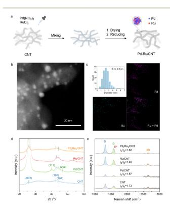
Fig. 1 (a) Schematic diagram of the 2 wt% Pd<sub>7</sub>Ru<sub>3</sub>/CNT preparation method, (b) STEM image of 2 wt% Pd7Ru3/CNT, (c) particle size distribution and elemental mapping of 2 wt% Pd<sub>7</sub>Ru<sub>3</sub>/CNT. (d) XRD analysis and (e) Raman spectra of CNT and the catalysts at 2% metal loading.
