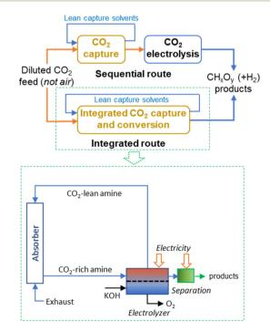
Fig. 2 Simplified block diagrams of sequential and integrated routes for amine-based  $CO_2$  capture and electrolysis with a more detailed scheme for the integrated  $CO_2$  capture and direct  $CO_2$  electroreduction from the capture medium. Some elements, such as the compression unit between the stripper and the electrolyser, are not shown.
