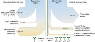
Fig. 10 Sankey diagrams of solar energy to plant- and algae-based food production compare the efficiencies of artificial and biological photosynthesis. Adapted from Hann et al. 182 Copyright Springer Nature 2022.
