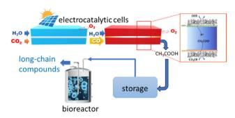
Fig. 8 In vitro artificial sugar synthesis system. CO2 was first converted to pure acetic acid through two-step electrolysis; this product was then directly fed for microorganism fermentation in a bioreactor to produce long-chain compounds, for example, glucose. In the inset: schematic illustration of CO reduction (COR) to pure acetic acid in the solid-electrolyte reactor. Original figure based on Zheng et al. 181 scheme.
