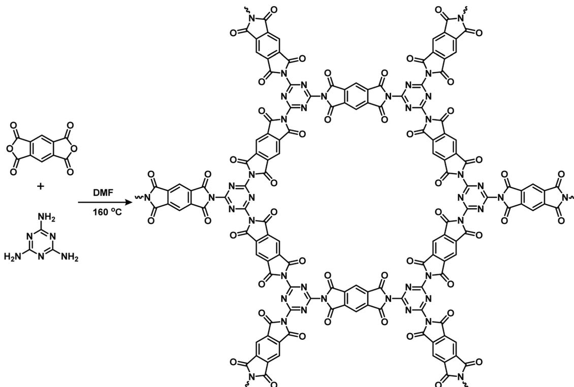
Scheme 1 Synthesis and chemical structure of TP-COF.
