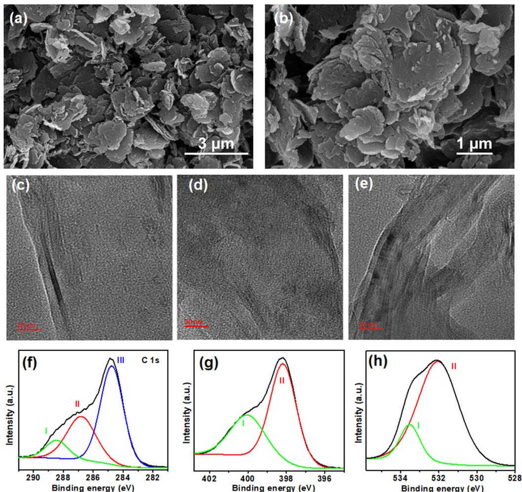
**Fig. 3** (a) and (b) The SEM images of TP-COF-C700 in different resolutions. The HRTEM images of (c) TP-COF-C600, (d) TP-COF-C700, and (e) TP-COF-C800. The core-level XPS spectra of (f) C 1s, (g) N 1s, and (h) O 1s of TP-COF-C700.
