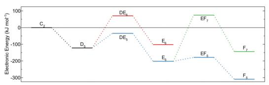
Fig. 6 Energy profile for TMA adsorption and decomposition on amino terminated AlN with a neighboring MMA fragment. The black step (C2 to D5) is adsorption of TMA. The blue path (D<sub>5</sub> to F<sub>5</sub>) is methyl protonation. The red path (D<sub>5</sub> to E<sub>6</sub>) is reductive elimination of the TMA adduct and the green path  $(E_5 \text{ to } F_7)$  is reductive elimination of the DMA fragment.
