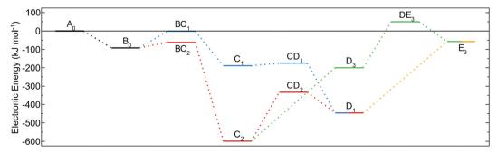
Fig. 3 Energy profile for TMA adsorption and decomposition on amino terminated AlN. The black step ( $A_0$  to  $B_0$ ) is initial adsorption of TMA. The blue path (Bo via C1 to D1) is methyl protonation followed by reductive elimination and red (Bo via C2 to D1) is reductive elimination followed by methyl protonation. The yellow path ( $D_1$  to  $E_3$ ) is surface oxidation, and the green ( $C_2$  via  $D_3$  to  $E_3$ ) is surface oxidation followed by methyl protonation.
