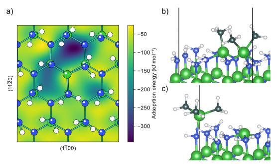
Fig. 5 Adsorption of TMA onto AlN with an aluminum adatom on the surface. (a) Potential energy surface for an adsorbing TMA molecule. (b) DMA fragment adsorbed after methyl transfer to aluminum adatom. (c) Structure of TMA adsorbing at an energy minimum forming a Lewis adduct.
