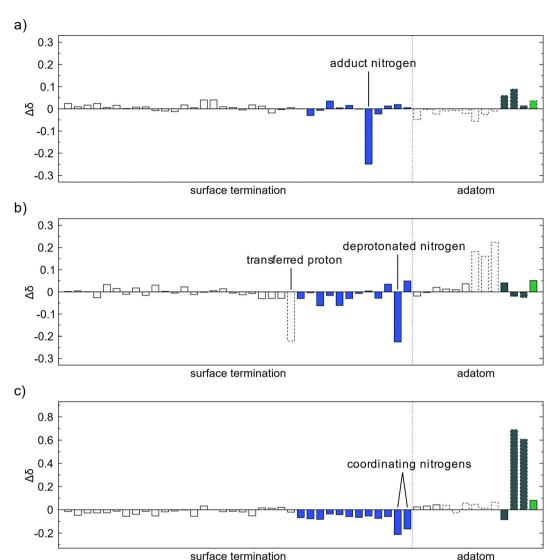
Fig. 7 Change of Bader charge after (a) TMA forms a Lewis adduct with an amino group, (b) methyl protonation, and (c) reductive elimination. The colors of the bars correspond to the element, white for hydrogen, blue for nitrogen, dark gray for carbon and green for aluminum. Bars with a dashed outline correspond to atoms adsorbing in (a) or desorbing in (b) and (c).
