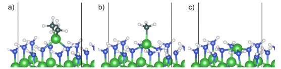
Fig. 2 Geometries for (a) DMA fragment after methyl protonation (C<sub>1</sub>), (b) MMA fragment after reductive elimination (C<sub>2</sub>) and (c) aluminum adatom after methyl protonation followed by reductive elimination ( $D_1$ ).
