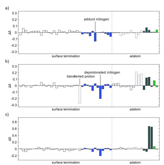
Fig. 8 Change of Bader charge on a surface with an MMA fragment after (a) TMA forms a Lewis adduct with an amino group, (b) methyl protonation, and (c) reductive elimination. The colors of the bars correspond to the element, white for hydrogen, blue for nitrogen, dark gray for carbon and green for aluminum. Bars with a dashed outline correspond to atoms adsorbing in (a) or desorbing in (b) and (c).
