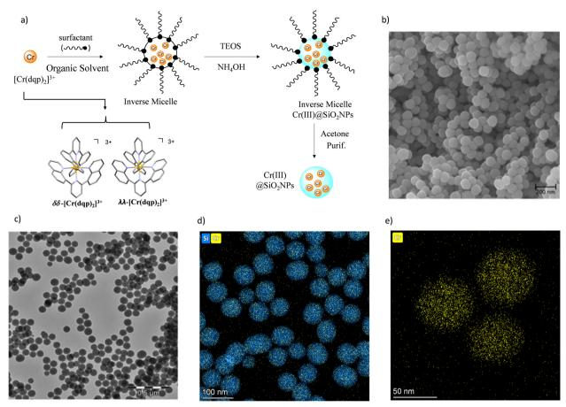
Fig. 3 (a) Schematic synthetic approach for preparing the silica nanoparticles (b) SEM image of the prepared rac-@SiO<sub>2</sub>NPs nanoparticles (c) TEM image of the prepared λλ-Cr@SiO<sub>2</sub>NPs; (d) and (e) HAADF-STEM compositional mapping image of λλ-Cr@SiO<sub>2</sub>NPs.
