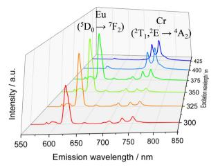
Fig. 7 Emission spectra for the  $(\lambda\lambda/\delta\delta)$ -EuCr $\alpha$ SiO $_2$ NPs under different excitation wavelength in ethanolic solution at room temperature.
