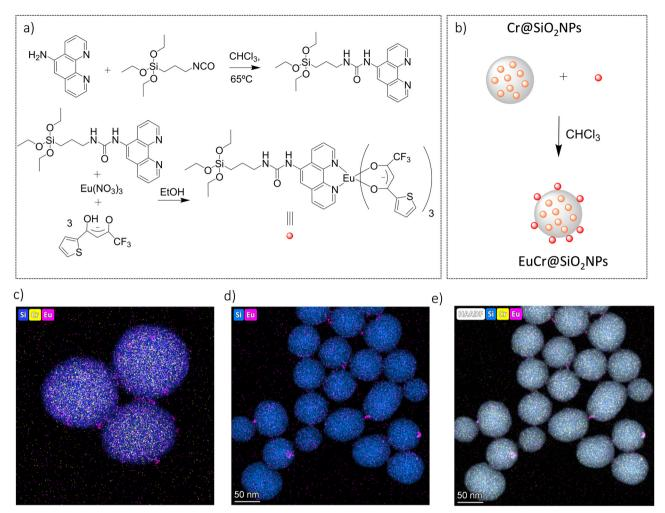
Fig. 6 (a) Synthetic steps for the preparation of the Eu<sup>III</sup> complex. (b) Schematic synthesis of  $(\lambda\lambda/\delta\delta)$ -EuCr@SiO<sub>2</sub>NPs (c) TEM image of the functionalized nanoparticle. (d) and (e) HAADF-STEM compositional mapping image of λλ-EuCr@SiO<sub>2</sub>NPs.
