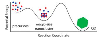
Fig. 4 Graphical representation illustrating MSCs as reaction intermediates in the synthesis of QDs. Figure adapted with permission from ref. 84. Copyright 2015 American Chemical Society
