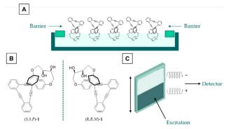
Fig. 1 Methodology of this work. (a) Langmuir – Schaefer films, (b) employed compounds and (c) CPL based barcoding design.
