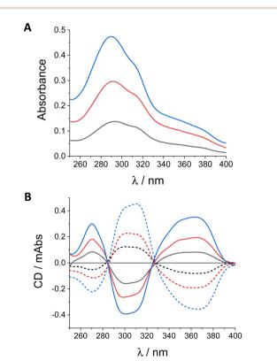
Fig. 6 (A) Absorbance and (B) CD spectra of (S,S,P)-1 (continuous lines) and (R,R,M)-1 (discontinuous lines) in quartz plates with 8 (black line), 16 (red line) and 32 (blue line) layers.
