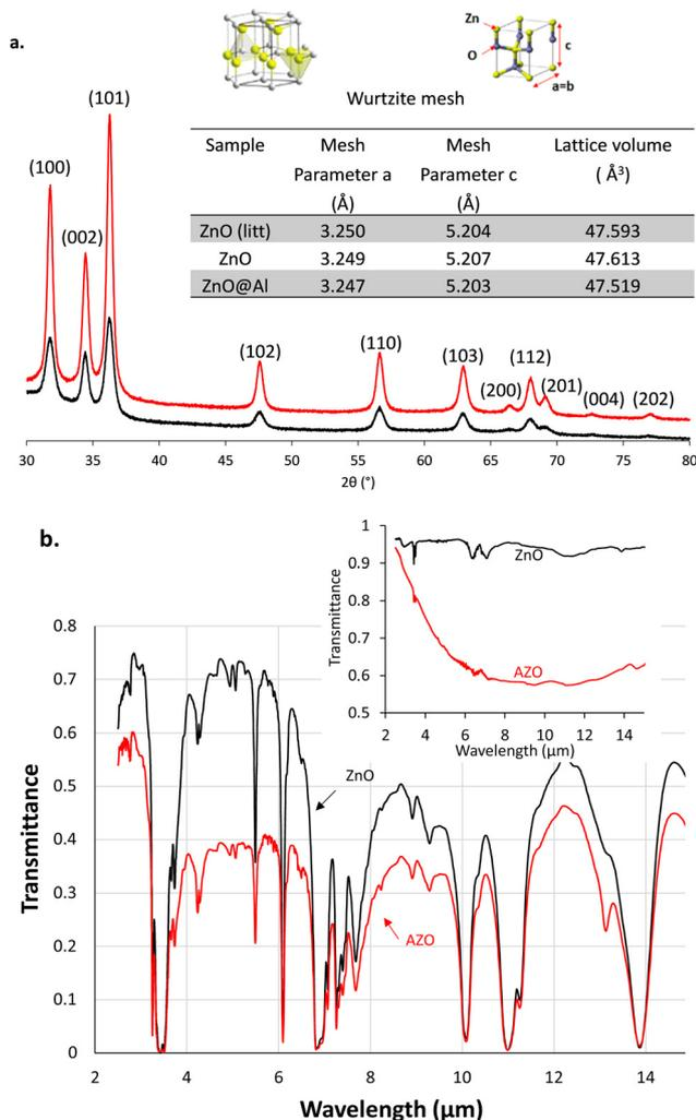
Fig. 2 (a) XRD measurement on AZO (in red) and ZnO (in black) nanocrystals. ZnO data from the literature<sup>43</sup> were used as a reference. (b) FT-IR spectrum of 8 mg L<sup>-1</sup> of AZO in HDE (red) and pur HDE (black). Inset: the IR-ATR spectrum of dried nanoparticles of AZO (red) and ZnO (black).
