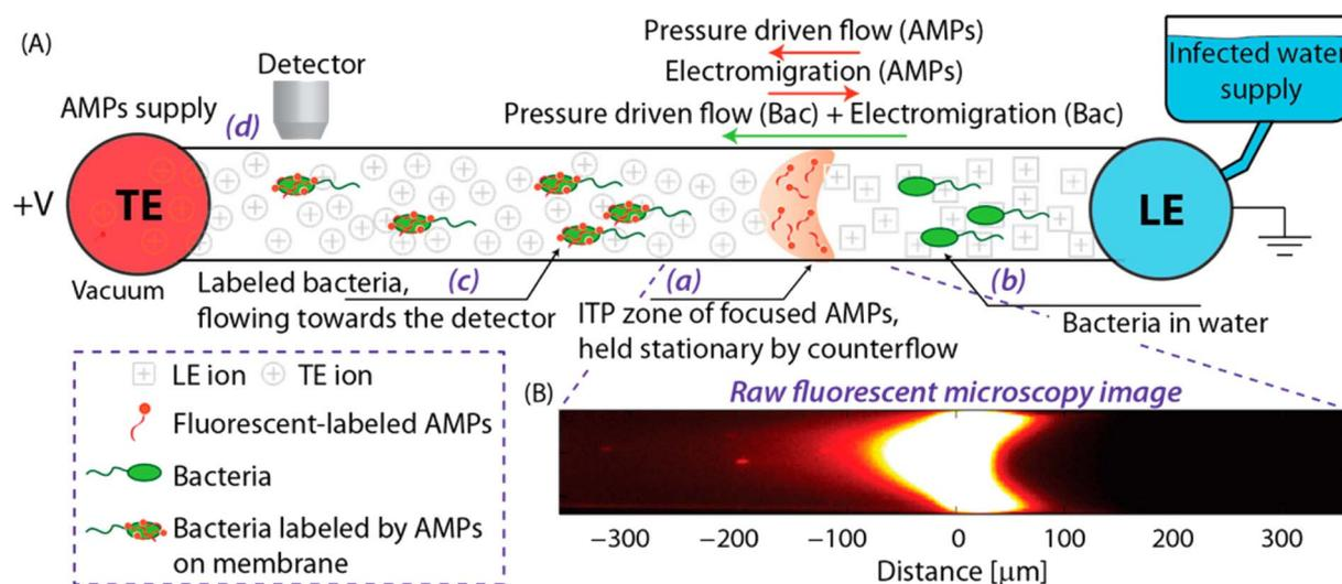
Fig. 1 (A) Schematic representation of the assay using a single straight channel, (B) fluorescently labelled *E. coli* at the highest concentration area.<sup>75</sup>
