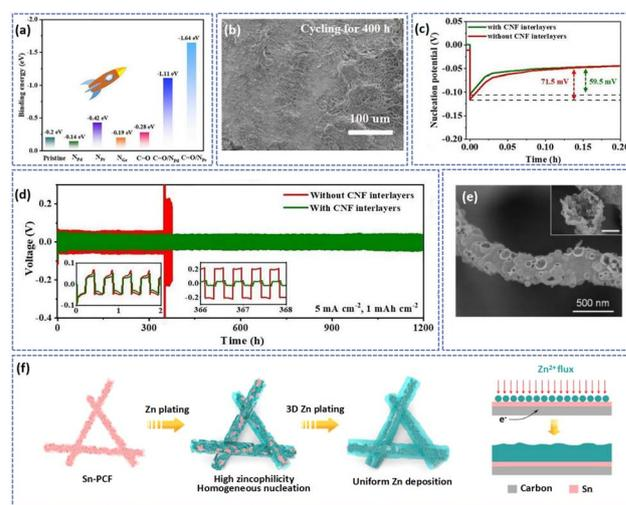
Fig. 8 (a) A comparison of the binding energy between Zn atoms and different adsorption sites. The morphology (b), charge/discharge curves (d), and Zn nucleation overpotential (c) at 5 mA cm<sup>-2</sup> with a capacity of 1 mA h cm<sup>-2</sup>. Adapted from ref. 33, copyright 2021, Elsevier B.V. (e) The SEM image and (f) Zn plating and nucleation diagrams on Sn-PCF. Adapted from ref. 134, copyright 2022, Elsevier B.V.
