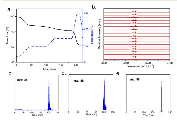
Fig. 4 TGA-FTIR-GCMS experiments on mmen-Mg<sub>2</sub>(dobpdc) with adsorbed  $CO_2$ : (a) thermogravimetric decomposition profile under humid He (black line); temperature ramp rate is shown in blue line; (b) FTIR spectra (0–50 min, 50–100 °C); characteristic  $CO_2$  was detected at 2360 and 2340 cm<sup>-1</sup>, each data was collected every 180 second. (c)–(e) gas chromatography mass spectra (GCMS) showing ions of released amine fragments.
