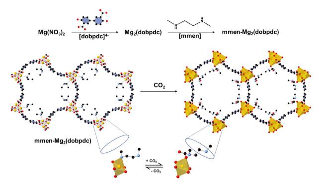
Fig. 1 Schematic illustration of diamine (mmen) appended Mg<sub>2</sub>(dobpdc) synthesis and structure. The framework structure is adopted from single crystal X-ray analysis of the isostructural zinc compound DEF-1. Yellow, red, and gray spheres represent Mq, O, and C atoms respectively; H atoms are omitted for clarity. Addition of mmen to the unsaturated framework yields the amine-appended Mg<sub>2</sub>(dobpdc). 17.22
