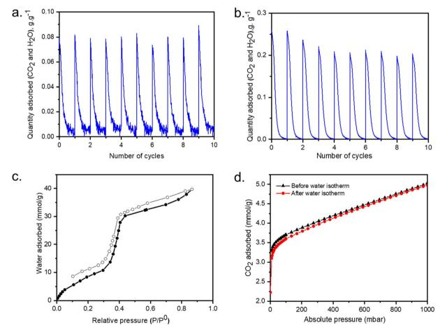
Fig. 5 Regeneration performance cycles at  $120 \,^{\circ}\text{C}$  for mmen-Mg<sub>2</sub>(dobpdc): (a) after exposing to ambient air with 25% relative humidity; (b) after exposing to ambient air with 45% relative humidity; (c) water isotherm at 25  $\,^{\circ}\text{C}$ ; (d) CO<sub>2</sub> adsorption isotherms before and after measuring water isotherms at 25  $\,^{\circ}\text{C}$ .
