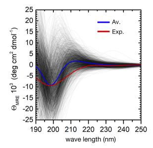
Fig. 4 Computation of the ensemble CD spectra of the peptide. Experimental CD spectrum (red curve) and simulated spectra (black lines) of 2000 conformers of the peptide in water. The blue curve is the calculated ensemble average
