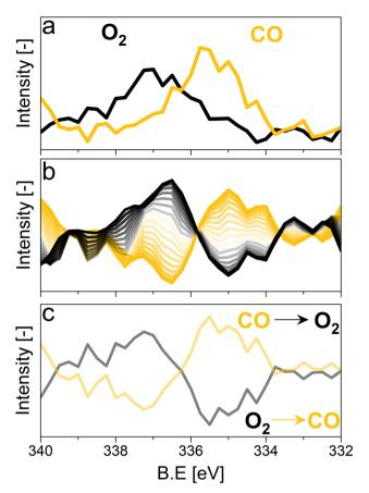
Fig. 4 (a) Average X-ray photoelectron spectra of 5 wt% Pd/Al $_2O_3$  at the Pd 3d core level with a 300 eV kinetic energy obtained 150 s after changing to the reducing and to oxidizing conditions. (b) Phase domain analysis performed on the smoothed data (binomial 1). (c) Difference spectra between the two boundary time-resolved spectra shown in the panel a. Only the Pd  $3d_{5/2}$  core level is shown.
