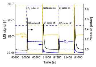
Fig. 2 Temporal behaviour of CO (yellow) and  $O_2$  (blue) MS signals as well as of the pressure in the experimental cell (black) during alternate  $O_2/CO$  pulsing. Pulses shape and timing is shown by the dashed lines.
