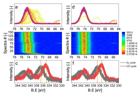
Fig. 3 X-ray photoelectron spectra of 5 wt%  $Pd/Al_2O_3$ . (a and b) and (d and e) Al 2p core level with a 650 eV kinetic energy. (b and e) Heat map of Al 2p core level spectra acquired during the 6 h measurement. (c and f) Pd 3d core level with a 300 eV kinetic energy. (a–c) Non-aligned spectra; (d–f) aligned spectra. The vertical lines in panels (c) and (f) correspond to the maximum intensity of the Pd 3d core level features in the  $O_2$  and CO periods.
