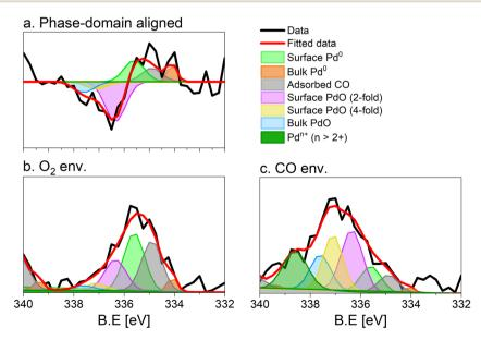
Fig. 5 Fit of the (a) phase (0°) and (b and c) time domain spectra ( $t = 150 \, \text{s}$ ), X-ray photoelectron spectra of 5 wt% Pd/Al<sub>2</sub>O<sub>3</sub> acquired at the Pd 3d core level. (b) Averaged spectrum in oxidising conditions, (c) averaged spectrum in reducing conditions. Peaks are defined in Table 1. Only the Pd 3d<sub>5/2</sub> core level is shown.
