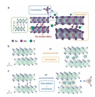
Fig. 1 (a) Schematic illustration of the modulation of Se–Se bonds. (b and c) Crystal structure and mechanism of  $MoSe_2$  and  $MoSe_{2+x}$ , respectively. Purple atoms represent selenium, pink atoms represent molybdenum, and green atoms represent potassium.
