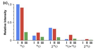
Fig. 8 Measurement using the oxygen isotope. (a) Mass spectra obtained under oxidized conditions for 5  $\mu$ M L-phosphatidylcholine (PC 18:1/18:1) in 500 mM HCl prepared using normal water (i) and water- $^{18}$ O (ii & iii). The operating gases are air (i & ii) and high-purity nitrogen (iii). Asterisk denotes the peak without oxidation. (b) Enlarged view of (a) (i) and (a) (ii). (c) Intensity comparison for different oxidation species.
