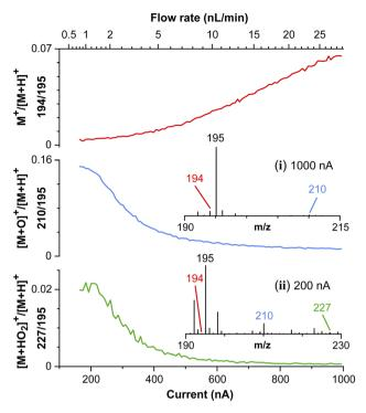
Fig. 5 Detection of caffeine molecular ion. Detection of caffeine (25  $\mu$ M) in 200 mM HCl under different spray currents. Red: Intensity ratio of M<sup>+</sup>/[M + H]<sup>+</sup>. Blue: [M + O]<sup>+</sup>/[M + H]<sup>+</sup>. Green: [M + HO<sub>2</sub>]<sup>+</sup>/[M + H]<sup>+</sup>. Mass spectra in the inset are taken at 1000 and 200 nA.
