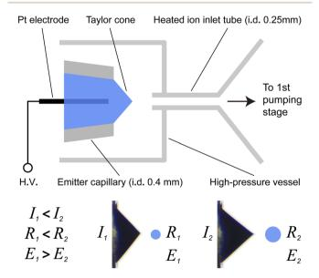
Fig. 1 Schematic of the offline high-pressure nanoESI ion source. The emitter capillary is a micropipette tip with an i. d. of 0.4 mm. The solution flow rate is determined from the measured spray current I. Insets show the shape of the Taylor cones formed at different flow rates. A lower flow rate produces a charged droplet of a smaller radius R with a higher electric field E.
