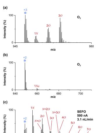
Fig. 7 Oxidation by ozone. (a) Oxidation of 10  $\mu$ M melittin in 100 mM ammonium formate using ozone produced from the DBD source. (b) Oxidation of 20  $\mu$ M angiotensin I in 50 mM HCl using ozone. (c) Strong electric field-induced oxidation of angiotensin I in 500 mM HCl. Asterisk denotes the unoxidized peak.
