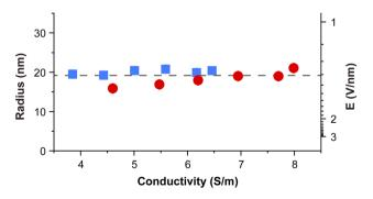
Fig. 4 Threshold electric field. Radius and the electric field of the initial droplet at the threshold for the detection of oxidized species. The sample is cytochrome c (25  $\mu\text{M}$ ) in different buffer solutions of various electrical conductivities. Blue square: ammonium acetate. Red circle: ammonium formate. The average threshold radius and electric field are  $\sim\!19.2$  nm and 1.3 V nm $^{-1}$ .
