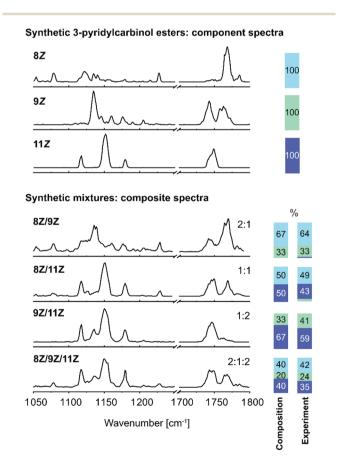
Fig. 2 Gas-phase infrared spectra of synthetic FA 18:1 (8Z), (9Z) and (11Z) 3-pyridylcarbinol ester standards and synthetic binary and ternary mixtures of known composition. Composite spectrum regression of the infrared spectra obtained from synthetic mixtures in the fingerprint and carbonyl stretching region yields the expected isomer contributions.
