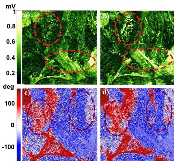
Fig. 3 PFM amplitude and phase images of a thin film of **1** on a  $5 \times 5 \mu\text{m}^2$  area; amplitude images of the (a) vertical and (b) lateral directions; and phase images of the (c) vertical and (d) lateral piezo-response.
