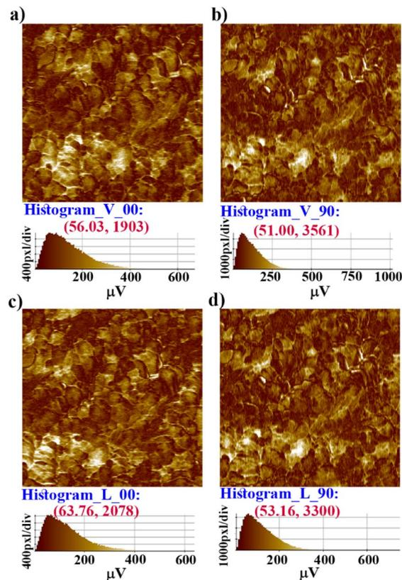
Fig. 4 PFM amplitude image of a crystalline thin film of **1**: (a) and (b) vertical and (c) and (d) lateral amplitude images collected by scanning the X and Y directions; the indication of 0 and 90 is relative. The corresponding histograms show that the maximum number of pixels have the most occurring amplitude value of deformation (in  $\mu\text{V}$ ).
