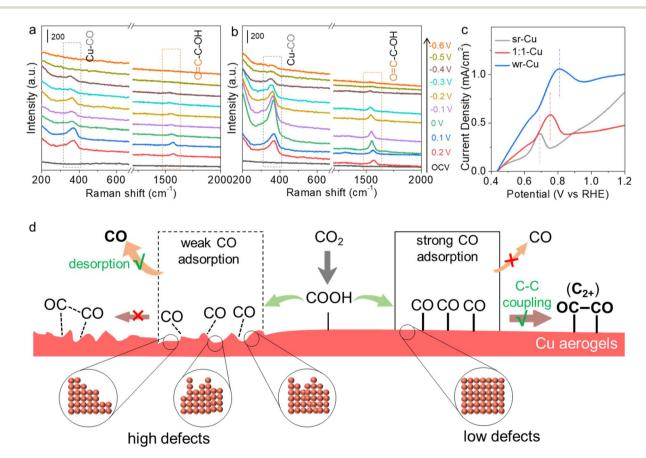
Fig. 3 The in situ Raman spectra for sr-Cu (a) and wr-Cu (b) aerogels at various potentials (vs. RHE) during the CO<sub>2</sub>RR. OCV means open-circuit voltage. (c) The electrochemical CO stripping voltammetry test for sr-Cu, 1:1-Cu and wr-Cu aerogels in CO-saturated 0.1 M Na<sub>2</sub>SO<sub>4</sub> solution. (d) Proposed structure—activity relationship diagram on different Cu aerogel surfaces: comparison of key steps in the C<sub>1</sub> and C<sub>2+</sub> reaction pathways.
