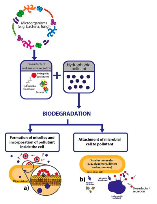
Fig. 6 Probable mechanistic actions of biosurfactants in the microbial decay of hydrophobic pollutants from soil media: (a) generation of micelles and encapsulation of organic contaminants within the microbial cell and (b) microbial attachment of hydrophobic pollutants. Reprinted with permission from ref. 95.
