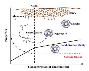
Fig. 5 Schematic representation of rhamnolipid-enhanced aqueous dispersion of HOCs. Reprinted with permission from ref. 82 Copyright 2018 Elsevier.
