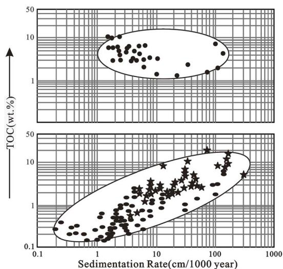
Fig. 3 Schematic comparison of sedimentation rate versus total organic carbon in sediments.<sup>66-69</sup>
