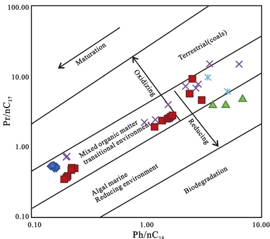
Fig. 10 Plot of Pr/*n*-C<sub>17</sub> against Ph/*n*-C<sub>18</sub> ratios of oils from Niger Delta.<sup>18,141</sup>
