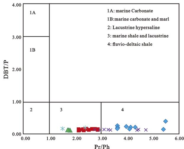
Fig. 14 A cross plot of dibenzothiophene/phenanthrene (DBT/P) and pristane/phytane (Pr/Ph) ratios for the Niger Delta oils.<sup>18,212</sup>
