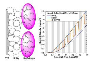
Fig. 14 LSV of KuQ3CO<sub>2</sub>H|meso-SnO<sub>2</sub> in aqueous ascorbate buffer pH 5.8, 20 mV s $^{-1}$ , light: AM 1.5G + 400 nm cut-off filter. Reproduced from ref 87
