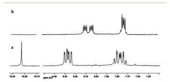
Fig. 4 Comparison between H-NMR spectra of KuQTEGMe in (a) CDCl<sub>3</sub>, (b) DMSO-d<sub>6</sub>. Reprinted with permission from ref. 27. Copyright 2017 American Chemical Society.
