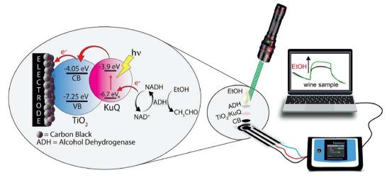
Fig. 15 Scheme of the photoelectrochemical sensing system and the experimental set-up for detection of ethanol. Reprinted from ref. 98. Copyright 2022, with permission from Elsevier
