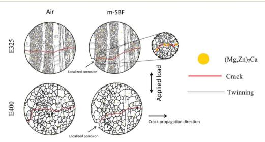
Fig. 12 Schematic diagram of fatigue cracking of ZX10 extruded at 325 °C and 400 °C when tested in air and m-SBF. 126
