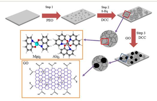
Fig. 25 Schematic diagram of the fabrication steps for GO/8-Hg/IC materials.<sup>248</sup>
