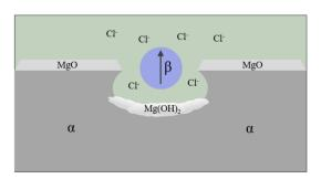
Fig. 7 Schematic of pitting corrosion. 131
