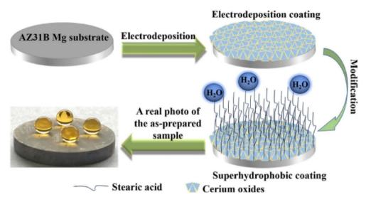
Fig. 28 Schematic diagram of preparation process of the superhydrophobic coating formed on the AZ31B Mg substrate.<sup>266</sup>
