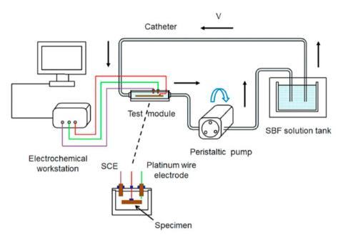
Fig. 16 Schematic diagram of a dynamic flow field test device. 181
