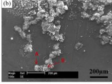
Fig. 10 Typical filamentary corrosion morphologies of Mg-3Zn immersed in 0.01 mol per L NaCl solution for 6 h at different scales (50  $\mu$ m and 200  $\mu$ m). <sup>121</sup>
