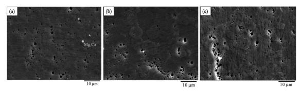
Fig. 18 SEM images of the (a) Mg-0.54Ca alloy; (b) Mg-0.79Ca alloy; (c) Mg-1.35Ca alloy. 198
