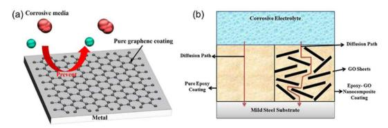
Fig. 22 (a) The graphene anti-corrosion coating.<sup>234</sup> (b) the "labyrinth effect" of GO enhanced epoxy resin coating.<sup>235</sup>
