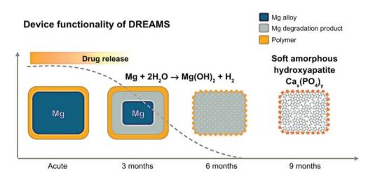
Fig. 4 Degradation model of DREAMS-2 stent.<sup>76</sup>
