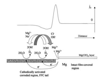
Fig. 9 Schematic representation of the mechanism of filiform corrosion under immersion conditions, showing how the regions of the localised corrosion cell correspond with empirically derived SVET  $j_z$  versus distance profiles.<sup>142</sup>
