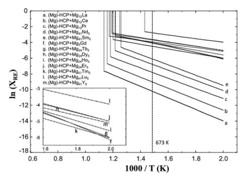
Fig. 21 Maximum solubility RE in hcp Mg in the binary Mg-RE alloy systems.<sup>225</sup>
