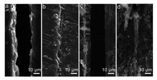
Fig. 29 SEM images of the (a) scratched SHEP coating, (b) healed SHEP coating, (c) healed PF-POS@silica coating, and (d) healed SHEP/PF-POS@silica coating.<sup>271</sup>
