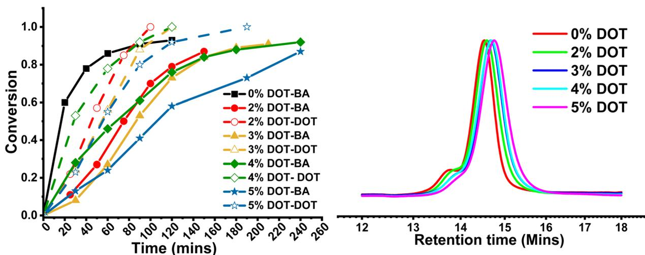
**Fig. 4** Left: Conversion plots for PBA-DOT-L linear polymers. Closed markers indicate BA conversion, open markers indicate DOT conversion. Right: GPC traces for PBA-DOT linear polymers after 24 h reaction time. [BA] : [DOT] : [DDMAT] : [AIBN] = 100 :  $x$  : 1 : 0.4,  $x = 0, 2, 3, 4, 5$ . BA : anisole 1 : 1 v/v, 65 °C.
