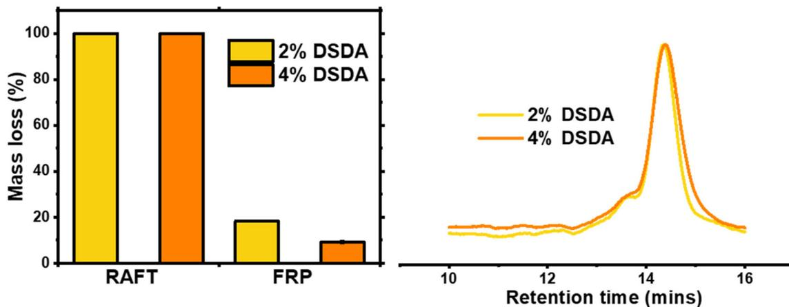
**Fig. 3** Degradation of PBA-DSDA gels by 25 mg mL<sup>-1</sup> DTT solution in DMF. Left: Mass loss % referenced to original mass of dry gel sample before degradation. 100% mass loss corresponds to macroscopic degradation of gel to soluble fragments. Right: GPC traces of soluble fragments from fully degraded PBA-DSDA RAFT networks.
