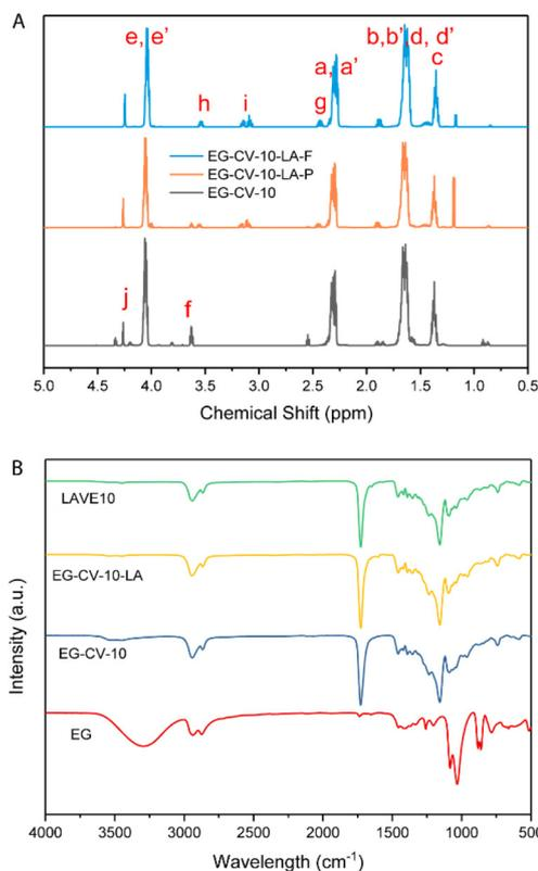
**Fig. 1** (A) <sup>1</sup>H-NMR spectra of EG-CV-10, EG-CV-10-LA-F (full substituted), and EG-CV-10-LA-P (partly substituted); (B) FTIR of EG, EG-CV-X, EG-CV-X-LA, and LAVE.
