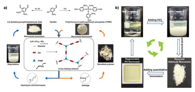
Fig. 3 (a) Synthetic route and reprocessing of the fully bio-based vitrimers. (b) Digital photographs of the chemical recycling process of PV-NDA-25 through the recovered monomer. Reproduced from ref. 114 with permission from the American Chemical Society, copyright 2022.
