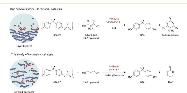
Fig. 1 Previous study on the depolymerisation of BPA-PC in bulk (interfacial catalysis) and the reaction presented in this study in appropriate solvent (volumetric catalysis).
