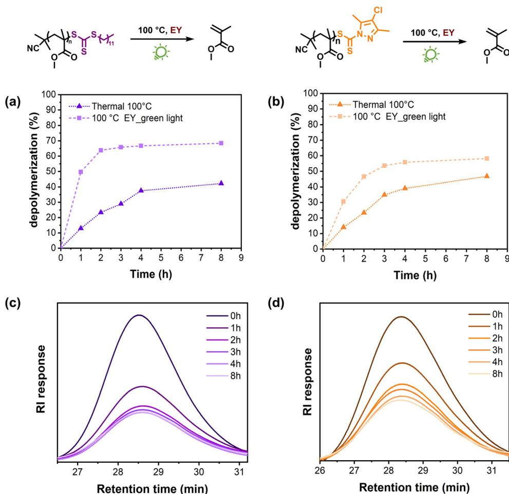
Fig. 3 Kinetic study comparing green light-accelerated depolymerization of PMMA catalysed by Eosin Y at 100 °C versus thermal depolymerization at 100 °C using (a) TTC and (b) pyrazoleCD chain transfer agents, respectively. SEC traces at different depolymerization times (c) and (d).
