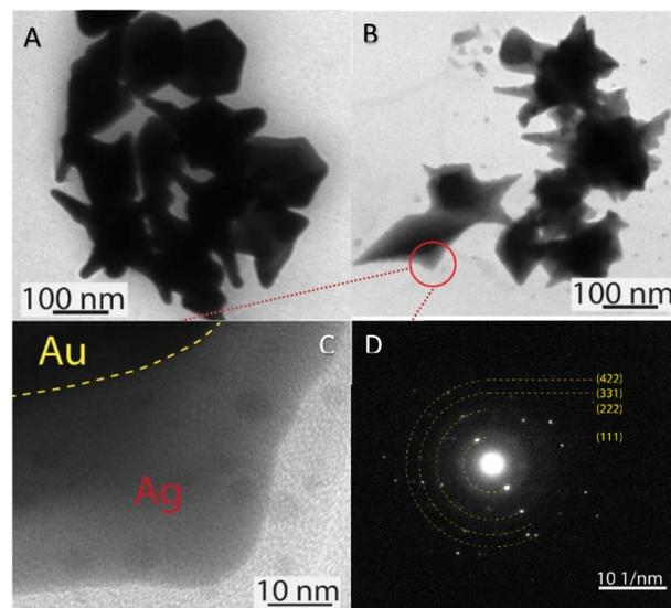
Fig. 4 TEM micrographs of AuNSs-CTAB@Ag with an average size of approximately 150 nm covered with (A) 150 and (B) 200 μL of AgNO<sub>3</sub>. (C) HRTEM image exhibiting contrast areas collected on the focus region of one particle reported in (B), revealing the Ag layer coverage on the Au core surface. (D) Selected area electron diffraction (SAED) pattern of AuNS-CTAB@Ag nanocrystal with bright spots, indicating that the formed nanoparticles were highly crystalline.
