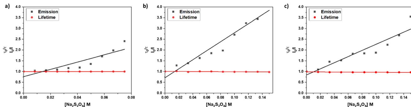
Fig. 7 Stern–Volmer quenching experiments for different systems: a) acetonitrile/water 1:1 (V:V), b) DOPG (14:0 PEG2000 PE):  $[1]^{2+} = 100:1:1$  liposomes in phosphate buffer (10 mM, pH 7.0) without size exclusion chromatography, c) DOPG (14:0 PEG2000 PE):  $[1]^{2+} = 100:1:1$  liposomes in phosphate buffer (10 mM, pH 7.0) after size exclusion chromatography.
