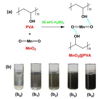
Fig. 1 (a) Interaction between MnO<sub>2</sub> and PVA. (b) Photo images of (b<sub>0</sub>) plane PVA, (b<sub>1</sub>) 1 wt% MnO<sub>2</sub>@PVA, (b<sub>2</sub>) 3 wt% MnO<sub>2</sub>@PVA, (b<sub>3</sub>) 5 wt%  $MnO_2@PVA$  and  $(b_4)$  7 wt%  $MnO_2@PVA$  gel electrolytes.
