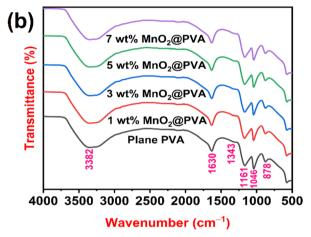
Fig. 2 FTIR spectra of (a)  $MnO_2$  powder, and (b) plane PVA and PVA loaded with different wt% of  $MnO_2$ .
