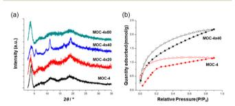
Fig. 7 (a) Powder XRD patterns of the MOC-4 and the supramolecular cross-linked products. (b) CO<sub>2</sub> adsorption experiments carried out at 195 K and 1.2 bar. Reproduced from ref. 52 with permission from ACS, copyright 2019
