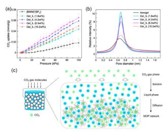
Fig. 5 (a)  $CO_2$  uptake isotherms of Gel\_IL at different concentrations of MOC-2 networks at 303 K under 100 kPa. (b) Particle size distribution of Gel\_IL with different concentrations of MOC-2 networks derived from PALS experiments. (c) Cartoon representing the  $CO_2$  gas diffusion pathway within the wet sample of connected MOCs. Reproduced from ref. 51 with permission from ACS, copyright 2023.
