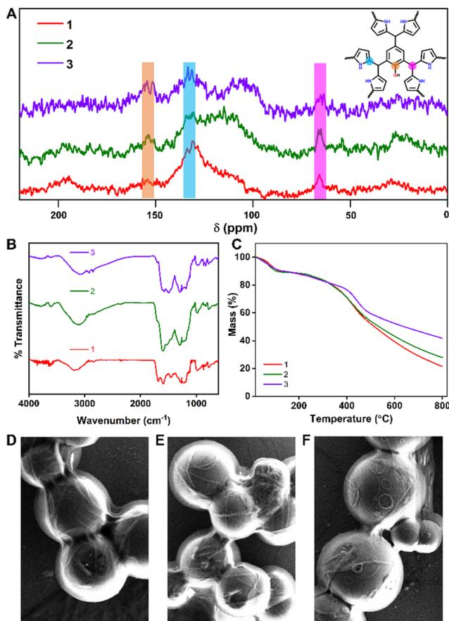
**Fig. 2** (A) Solid state NMR of POFs showing the characteristic peaks. (B) IR-spectra of the POFs showing the peaks corresponding to the different stretching frequencies. (C) Thermo-gravimetric analysis of the POFs showing the high thermal stability. (D)–(F) FE-SEM morphology of 1, 2 and 3 respectively. (SEM images with the scale bar are shown in the ESI†).
