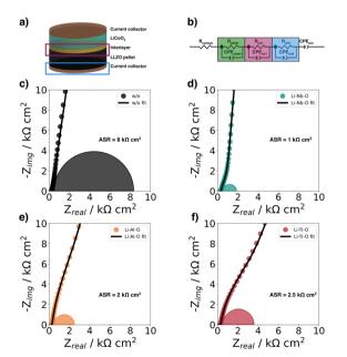
Fig. 5 (a) Schematic of half-cells structure for electrochemical impedance spectroscopy at room-temperature, (b) equivalent circuit model used to fit the impedance spectra by Zhang et al., 43 EIS spectra of (c) Au|LCO|LLZO|Au (w/o), (d) Au|LCO|Li-Nb-O|LLZO|Au (Li-Nb-O), (e) Au|LCO|Li-Al-O|LLZO|Au (Li-Al-O), and f) Au|LCO|Li-Ti-O|LLZO|Au (Li-Ti-O). The measured data are shown together with the fits from the equivalent circuit
