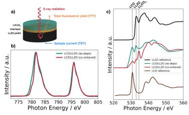
Fig. 3 (a) Schematic of the XAS measurement geometry, (b) Co L<sub>2,3</sub>-edge, and (c) O K-edge in fluorescence mode (TFY) for LLZO, LCO, and 50 nm LCO|LLZO as-deposited and annealed at 500 °C in oxygen.
