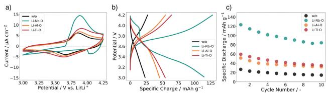
Fig. 6 (a) Cyclic voltammetry scans measured with a sampling rate of  $0.1 \text{ mV s}^{-1}$  between 3 and  $4.25 \text{ V vs. Li/Li}^+$ , (b) charge–discharge curves with 1.75  $\mu$ A cm<sup>-2</sup> between 3 V and 4.2 V at 80 °C, and (c) specific discharge capacities for full cells with and without interface modification.
