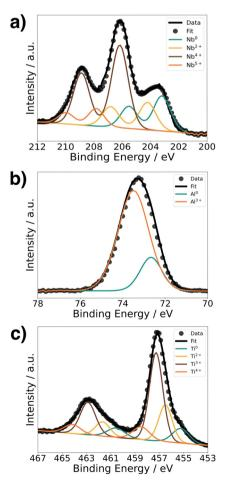
Fig. 1 XPS spectra of the core-level metal elements for (a) Li-Nb-O, (b) Li-Al-O, and (c) Li-Ti-O.
