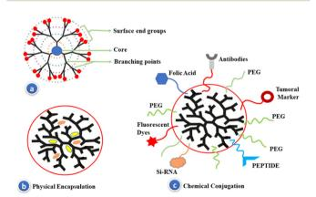
(a) Primary structural properties of dendrimers (b) dendrimer nanocarriers wherein the active components (including drug molecules) are entrapped within the internal cavity of dendrimers; (c) or conjugation to their surface-functionalized groups
