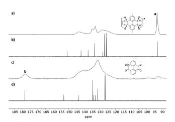
Fig. 4  $^{13}$ C CP MAS NMR spectra (10 000 Hz) of **D-PTK 2** (a), **D-PTO 2a** (c) and  $^{13}$ C NMR spectra (CDCl<sub>3</sub>, 150 MHz) of model compounds **1** (b) and **2** (d).
