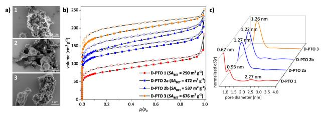
Fig. 5 (a) SEM images of **D-PTO-1**, **-2a**, and **-3** (from top to bottom). (b) BET gas sorption isotherms ( $N_2$ , 77 K, vector dosing) after activation at 120 °C for 12 h. (c) pore size distribution (QSDFT, Kernel:  $N_2$  on carbon at 77 K, sphere/cylindrical pore.
