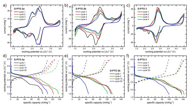
Fig. 6 Electrochemical performance of composite electrodes of D-PTO 2a, 2b and 3 (vs. Li/Li<sup>+</sup> and TFSI as electrolyte): (a-c) cyclic voltammograms obtained at a scan rate of 0.1 mV s<sup>-1</sup>. (d-f) Galvanostatic charge and discharge profiles for cycling at 100 mA g<sup>-1</sup>
