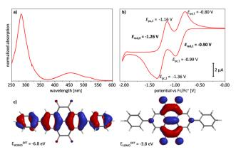
Fig. 2 (a) UV/Vis spectrum of compound 2 measured in  $CH_2Cl_2$  at rt (1  $\mu$ mol L<sup>-1</sup>). (b) Cyclic voltammogram of model compound **2** (CH<sub>2</sub>Cl<sub>2</sub>, nBu<sub>4</sub>NPF<sub>6</sub> (0.1 M), measured at rt with Pt-working electrode and (Fc/Fc+) as internal reference, scanning velocity:  $100 \text{ mV s}^{-1}$ ). (c) DFT model (B3LYP: 6-311++G\*\*) of compound 2 (tert-butyl groups omitted).
