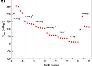
**Fig. 7** Electrochemical performance of **D-PTO-2a** based composite electrodes within the potential range of  $1.5-4~V~(vs.~Li/Li^+)$ : (a) cycling performance at 100 mA  $g^{-1}$ . (b) Rate performance at various current densities.
