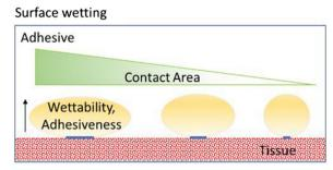
Fig. 4 Surface wetting is considered an important contributor to adhesiveness. If the adhesive makes extended molecular contact with the tissue surface, the contact angle will be close to zero, resulting in high-quality wetting and an adhesive effect. Reproduced from Biomater. Sci., 2020, 8, 1240-1255 with permission from the Royal Society of Chemistry.
