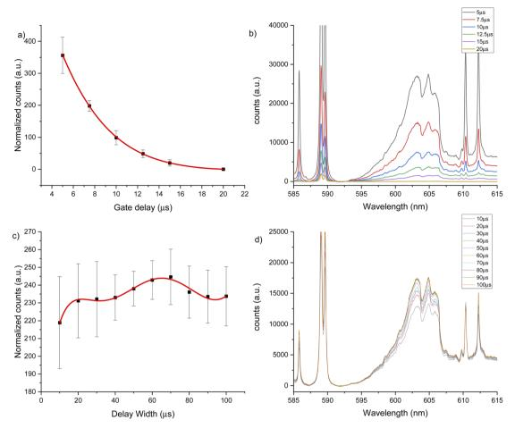
Fig. 5 LIBS signal optimization under helium flow of  $1 \text{ L min}^{-1}$  for 600 nm window using a 2500 μg g<sup>-1</sup> hydroxyapatite standard. (a) Gate delay optimization maintaining constant gate width at 50 μs, (b) LIBS spectrum for each gate delay change, (c) gate width optimization maintaining constant gate delay at 10 μs, (d) LIBS spectrum for each gate width change.
