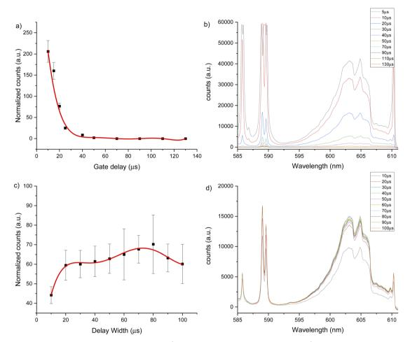
Fig. 4 LIBS signal optimization under argon flow of  $1 \, \text{L} \, \text{min}^{-1}$  for 600 nm window using a 2500 μg g<sup>-1</sup> hydroxyapatite standard. (a) Gate delay optimization maintaining constant gate width at 50 μs, (b) LIBS spectrum for each gate delay change, (c) gate width optimization maintaining constant gate delay at 20 μs, (d) LIBS spectrum for each gate width change.
