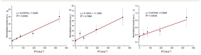
Fig. 7 Calibration curve for CaF LIBS signal under argon gas flow for three different spectral windows, (a) 530 nm, (b) 600 nm and (c) 689 nm.
