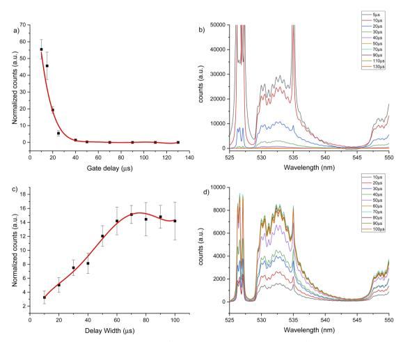
Fig. 2 LIBS signal optimization under argon flow of  $1 \, \text{L min}^{-1}$  for 530 nm window using a 2500  $\mu g \, g^{-1}$  hydroxyapatite standard. (a) Gate delay optimization maintaining constant gate width at 50  $\mu s$ , (b) LIBS spectrum for each gate delay change, (c) gate width optimization maintaining constant gate delay at 20  $\mu s$ , (d) LIBS spectrum for each gate width change.
