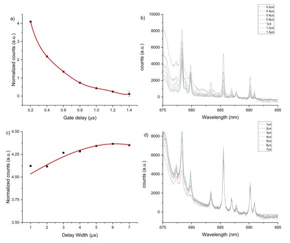
Fig. 6 LIBS signal optimization under helium flow of  $1 \, \text{L} \, \text{min}^{-1}$  for 689 nm window using a 2500 μg g<sup>-1</sup> hydroxyapatite standard. (a) Gate delay optimization maintaining constant gate width at 4 μs, (b) LIBS spectrum for each gate delay change, (c) gate width optimization maintaining constant gate delay at 0.2 μs, (d) LIBS spectrum for each gate width change. Error bars on (a) and (c) are too small to be seen.
