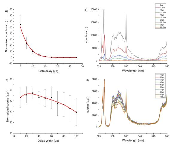
Fig. 3 LIBS signal optimization under helium flow of  $1 \text{ L min}^{-1}$  for 530 nm window using a 2500  $\mu$ g g<sup>-1</sup> hydroxyapatite standard. (a) Gate delay optimization maintaining constant gate width at 50  $\mu$ s, (b) LIBS spectrum for each gate delay change, (c) gate width optimization maintaining constant gate delay at 10  $\mu$ s, (d) LIBS spectrum for each gate width change.
