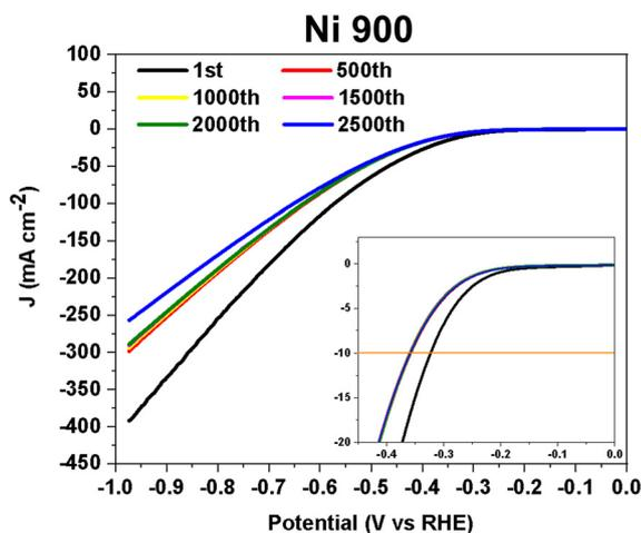
**Fig. 10** HER stability test (2500 cycles) on the Ni 900 electrocatalyst.
