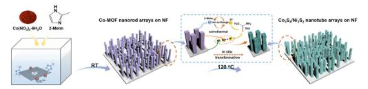
Fig. 1 Transformation of Co-MOF nanorod arrays on nickel foam into  $Co_3S_4$ -Ni $_3S_2$  nanotube arrays using ethanol with thioacetamide (TAA) under solvothermal conditions showing Ni $^{2+}$  exfoliation, ion–ion reaction, ionic exchange and doping mechanisms that cause simultaneous Co-MOF nanorod decay and  $Co_3S_4$ -Ni $_3S_2$  nanotube growth.
