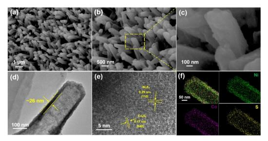
Fig. 2  $Co_3S_4/Ni_3S_2$ -3 nanotube arrays obtained after solvothermal sulfurization: (a–c) SEM images with different magnifications, (d) TEM image, (e) HRTEM image and (f) TEM-EDS elemental mappings.
