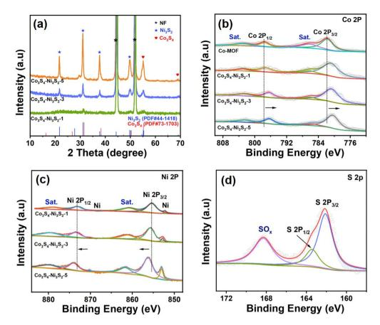
Fig. 3 (a) XRD patterns of the as-prepared  $Co_3S_4/Ni_3S_2$ -t materials at different sulfurization times (t = 1 h, 3 h, and 5 h). (b) Co 2p XPS region, (c) Ni 2p XPS region and (d) S 2p XPS region.
