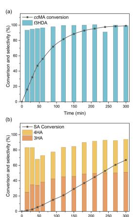
**Fig. 6** Conversion and selectivity achieved for the bulk electrolysis of (a) *cis,cis*-muconic acid (*cc*MA), and (b) sorbic acid (SA) in a divided flow reactor operated at a constant current of 100 mA cm<sup>-2</sup>. *cc*MA only produced *trans*-3-hexenedioic acid (*t*3HDA) while SA produced 3-hexenoic acid (3HA) and 4-hexenoic acid (4HA)
