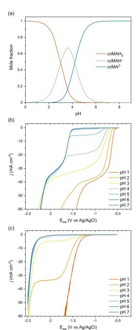
**Fig. 2** (a) Speciation diagram for ccMA calculated for  $pK_{a_1} = 3.0$  and  $pK_{a_2} = 4.2$ ;  $ccMAH_2$ ,  $ccMAH^-$ , and  $ccMA^{2-}$  correspond to diprotic, monoprotic, and fully deprotonated species. (b and c) pH-Dependent current–potential polarization curves on Pb RDE for 0.1 M K<sub>2</sub>SO<sub>4</sub>/H<sub>2</sub>SO<sub>4</sub> (b) with 0.5 g L<sup>-1</sup> ccMA and (c) without ccMA.
