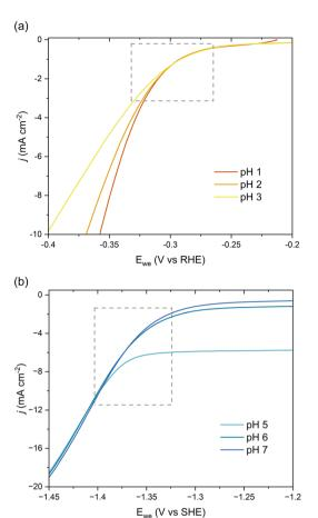
Fig. 3 pH-Dependent current–potential polarization curves on Pb RDE for 0.5 g  $\rm L^{-1}$  ccMA relative to (a) RHE and (b) SHE scales.
