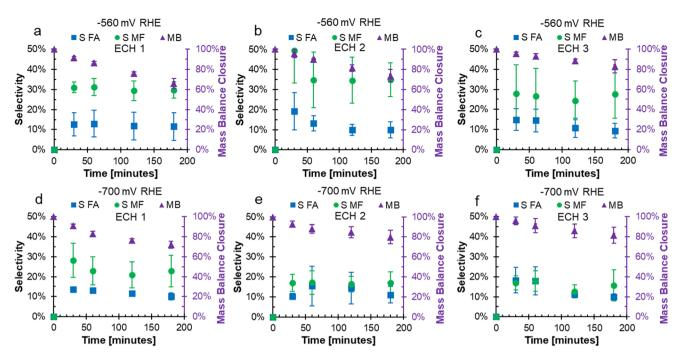
Fig. 2 Mass balance and selectivity to FA and MF from consecutive ECH of FF with recycled Cu foil electrode. At -560 mV RHE: (a) ECH1, (b) ECH2, (c) ECH3. At -700 mV RHE: (d) ECH1, (e) ECH3. Conditions: 200 mM FF, 0.5 M H<sub>2</sub>SO<sub>4</sub>, 80: 20 vol% water: acetonitrile, 3 hours duration ECH, 60 mL N<sub>2</sub> sparging, Cu electrode.
