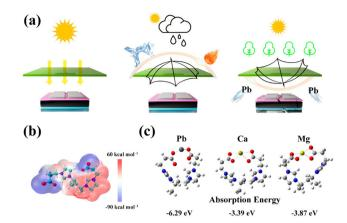
Fig. 12 (a) Ambidextrous protective shield manufactured by PPVI-TFSI. (b) Electrostatic potential distribution for PPVI-TFSI. (c) Optimized structures and absorption energy for PIL toward different cations. Reproduced from ref. 41 with permission from ACS, 2023.
