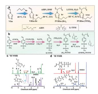
**Fig. 16** Synthesis and characterization of two poly(ionic liquids). (a) Synthetic scheme of PVBIm·(TFSI)<sub>n</sub>. (b) Synthetic scheme of (EMIM)<sub>n</sub>·PSTFSI. (c) <sup>1</sup>H NMR for VBIm·Br and PVBIm·(TFSI)<sub>n</sub>. (d) <sup>1</sup>H NMR for K·STFSI and (EMIM)<sub>n</sub>·PSTFSI. Reproduced from ref. 54 with permission from Wiley, 2021.
