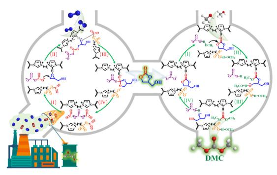
Fig. 9 Catalytic mechanism of diluted CO<sub>2</sub> coupling reaction. Reproduced from ref. 22 with permission from Elsevier, 2023.
