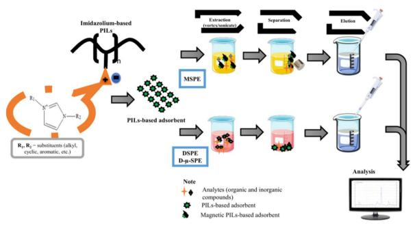
Fig. 18 The general scheme of analytical approaches using imidazolium PILs described in ref. 6. Reproduced from ref. 6 with permission from Elsevier, 2023.
