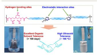
**Fig. 22** The interfacial adhesion to a combination of electrostatic interactions and hydrogen bonds, obtained from Deng *et al.*<sup>75</sup> Reproduced from ref. 75 with permission from ACS, 2022.
