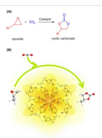
Fig. 7 (A) Synthesis of cyclic carbonates from CO<sub>2</sub> and epoxides. Reproduced from ref. 19 with permission from CSIRO Publisher, 2021. (B) Schematic representation of CO<sub>2</sub> capture with the participation of poly(ionic liquid)s with high ionic density (HDPILs). Reproduced from ref. 20 with permission from Wiley, 2023.
