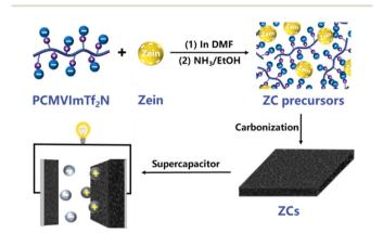
**Fig. 17** Scheme of fabrication and application of the eco-friendly supercapacitor using PIL. Reproduced from ref. 59 with permission from Elsevier, 2023.
