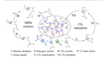
Fig. 8 Mechanism diagram of the cycloaddition reaction between glycidyl and CO<sub>2</sub> catalyzed by P-DVB-CE/CCImCl. Reproduced from ref. 21 with permission from Elsevier, 2023.
