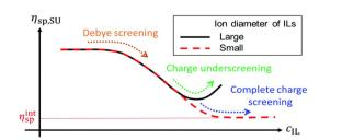
Fig. 20 The dependence of the specific viscosity (on the Y axis) against ion concentration of IL or PIL (on the X axis) obtained from the resulting equation in ref. 71. Reproduced from ref. 71 with permission from The Royal Society of Chemistry, 2022.
