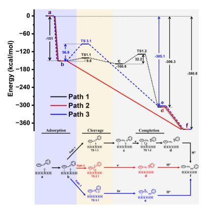
Fig. 6 Relative free energy diagram for C-O bond cleavage in BPE by a Ni catalyst (upper sector); proposed pathways for the catalytic C-O bond cleavage (lower sector).
