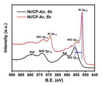
Fig. 2 XPS comparison between Ni/CP-Air (black line) & Ni/CP-Ar (red line). The Ni/CP-Air electrode was prepared under air atmosphere & the CP was undergone 5 h electroplating in 40 mM of NiCl $_2$ ·6H $_2$ O in methanol at 10 mA. The Ni/CP-Ar electrode was prepared under Ar atmosphere & the CP was undergone 5 h electroplating in 40 mM of NiCl $_2$ ·6H $_2$ O in methanol at 10 mA.
