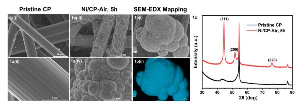
Fig. 1 (a) (i δii) SEM images of pristine carbon paper (CP); (iii δ iv) CP after electroplating from a 40 mM solution of NiCl<sub>2</sub>·6H<sub>2</sub>O for 5 h under air (Ni/CP-Air); (b) (i δii) SEM δEDX elemental mapping of Ni/CP-Air; (c) XRD spectrum of pristine CP δ Ni/CP-Air.
