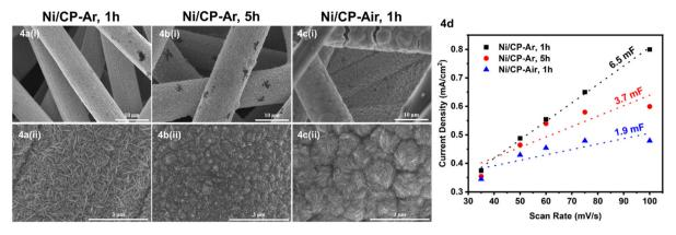
Fig. 4 (a) (i & ii) SEM images of the Ni/CP-Ar, 1 h; (b) (i & ii) Ni/CP-Ar, 5 h; (c) (i & ii) Ni/CP-Air, 1 h; (d) double-layer charging current vs. scan rate of Ni/CP-Ar, 1 h; Ni/CP-Ar, 5 h; Ni/CP-Air, 1 h. The linear slope is equivalent to the double-layer capacitance  $(C_{\rm dl})$ .
