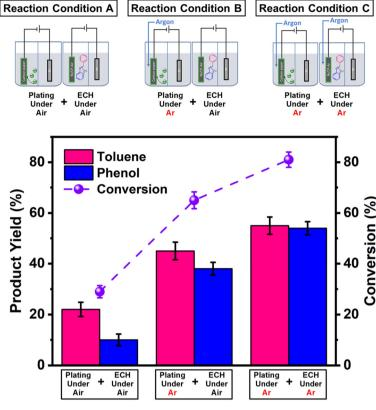
Scheme 1 Top: schematic representation of the plating atmosphere (air or argon; left side) and ECH atmosphere (air or argon; right side) combinations; bottom: product yields and conversion for ECH carried out under the three outlined conditions above.
