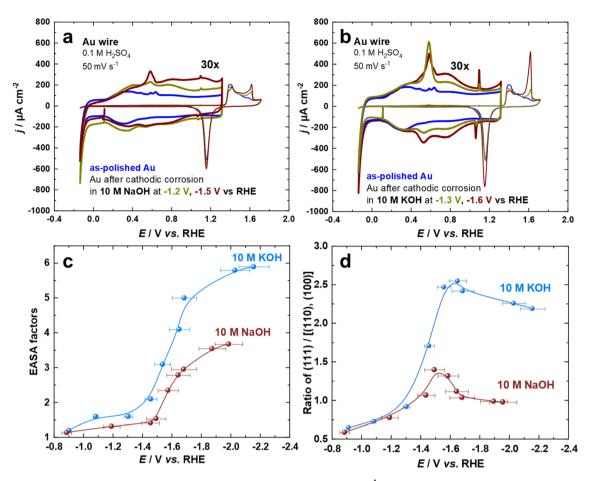
Fig. 1 Cyclic voltammograms for Au electrodes in 0.1 M  $H_2SO_4$  at a scan rate of 50 mV  $s^{-1}$  before and after cathodic polarization in (a) 10 M NaOH and (b) 10 M KOH at different applied potentials vs. RHE for 60 s. The current scale of the double-layer region is amplified 30 times. (c) Calculated EASA factors and (d) ratio of (111)/[(110), (100)] surface facets.
