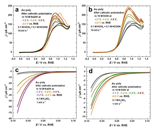
Fig. 5 Current–potential curves of Au electrodes in 0.1 M HClO<sub>4</sub> + 0.1 M HCOOH at a scan rate of 10 mV s<sup>-1</sup> before and after polarization in (a) 10 M NaOH and (b) 10 M KOH at various potentials for 60 s. Current–potential curves of Au electrodes in 0.1 M H<sub>2</sub>SO<sub>4</sub> at a scan rate of 1 mV s<sup>-1</sup> before and after polarization in (c) 10 M NaOH and (d) 10 M KOH at different potentials for 60 s. The current in a–d is normalized to the EASA.
