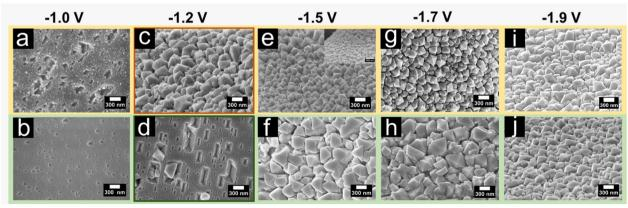
Fig. 3 SEM micrographs of Au electrodes after cathodic polarization in 10 M NaOH for 60 s at (a and b) -1.0 V, (c and d) -1.2 V, (e and f) -1.5 V, (g and h) -1.7 V, and (i and j) -1.9 V vs. RHE. The scale bar in the SEM images is 300 nm. A schematic illustrating the local structure of the corroded wire is illustrated above the SEM micrographs.
