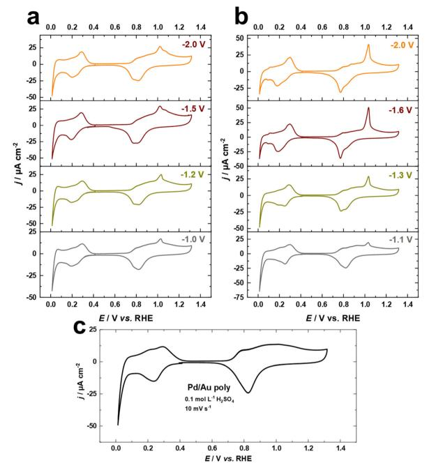
Fig. 6 Current-potential curves for Pd overlayers on (a and b) cathodically corroded and (c) as-polished Au electrodes in 0.1 M H<sub>2</sub>SO<sub>4</sub> at a scan rate of 50 mV s $^{-1}$ . The Au electrodes were cathodically corroded for 60 s in (a) 10 M NaOH and (b) 10 M KOH before Pd deposition from a chloridecontaining solution.
