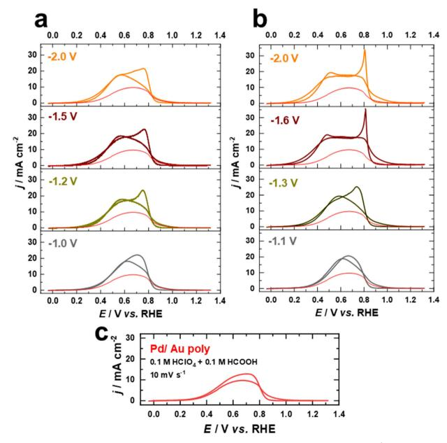
Fig. 7 Current-potential curves of Pd films on Au electrodes in 0.1 M  $HClO_4 + 0.1$  M HCOOH at a scan rate of 10 mV s<sup>-1</sup>. The Au electrodes were cathodically polarized in (a) 10 M NaOH and (b) 10 M KOH at various potentials for 60 s compared to (c) an as polished Au electrode.
