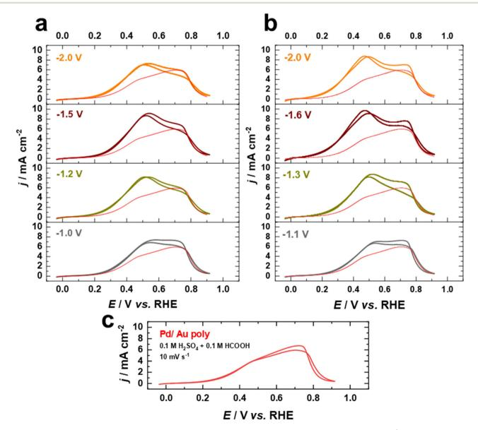
Fig. 8 Current-potential curves of Pd films on Au electrodes in 0.1 M  $H_2SO_4 + 0.1$  M HCOOH at a scan rate of 10 mV s<sup>-1</sup>. The Au electrodes were cathodically polarized in (a) 10 M NaOH and (b) 10 M KOH at various potentials for 60 s compared to (c) an as polished Au electrode.
